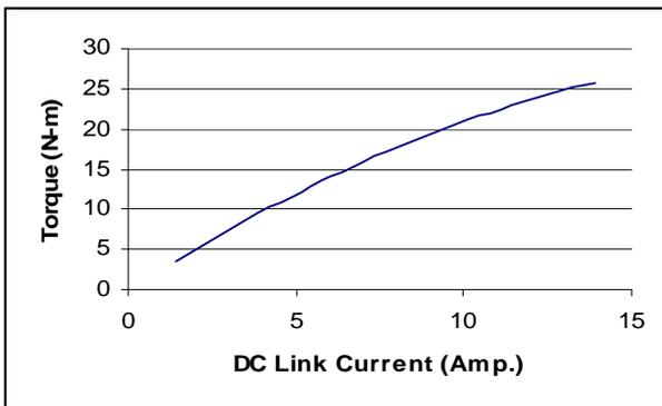
Fig. 7: Torque versus DC link current characteristics.
