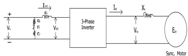
**Fig. 2:** Equivalent circuit diagram of commutatorless motor.
