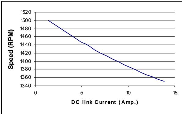
Fig. 6: Speed versus DC link current characteristics.
