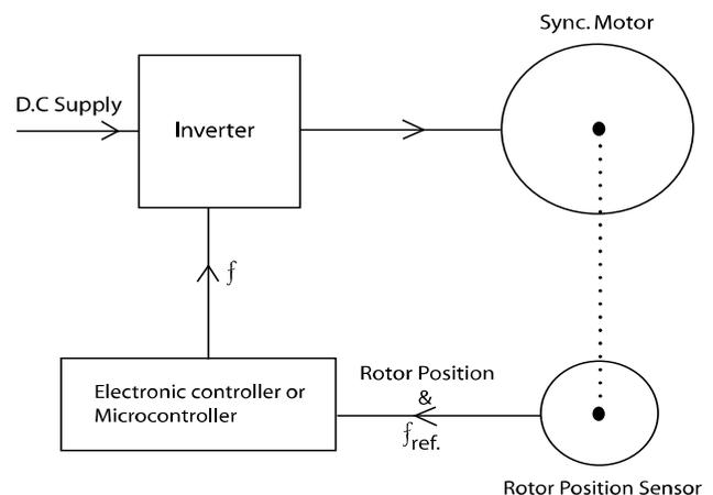
Fig. 1: Block diagram of commutatorless DC shunt motor.
