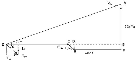
**Fig. 3:** Vector diagram of commutatorless DC motor.
