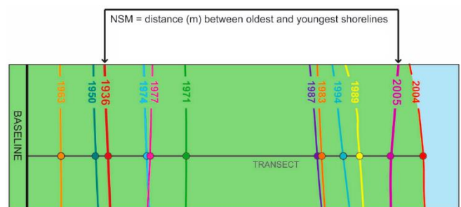
Fig. 7: A Bankline dataset including baseline (black), transect (gray), and shoreline and intersect data (multicolor) to illustrate the relationship between net Bankline movement
