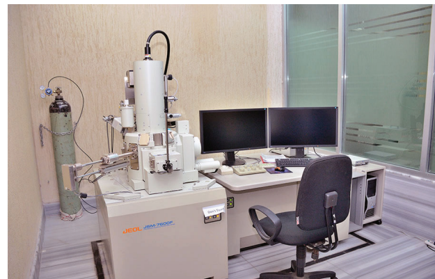
Fig. 5: SEM analysis machine used for this study (Model: JSM 7600F, JEOL-JAPAN)
