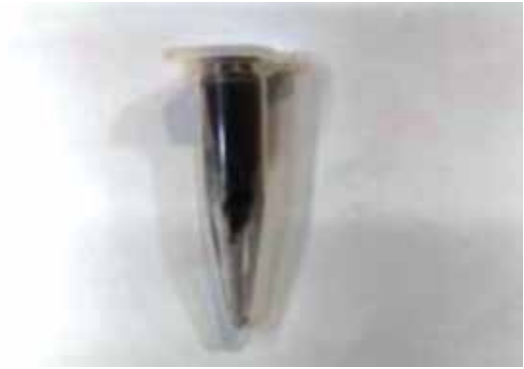
Fig. 4: Dried powder form of the synthesized \text{Fe}_3\text{O}_4 magnetic nanoparticles obtained after vacuum filtration and oven drying.
